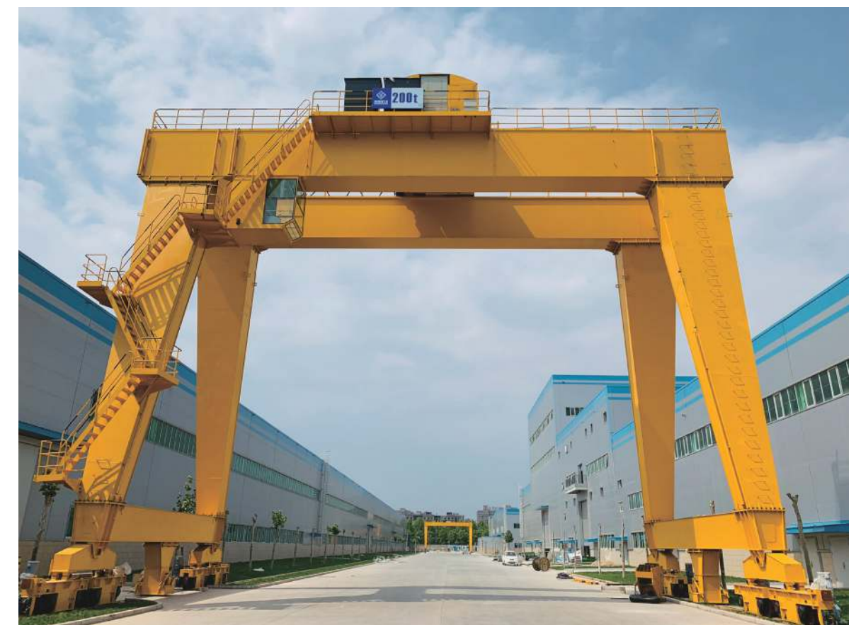
双梁门式起重机 Double-beam Gantry Crane
