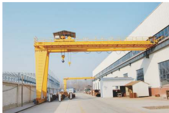
MGB double-girder semi-gantry crane with hook
