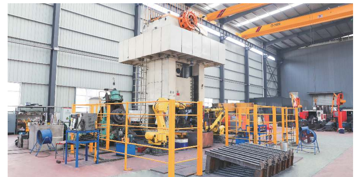
车轮锻造碾压复合工艺智能化流水线 Intelligent assembly line of wheel forging and rolling composite process
