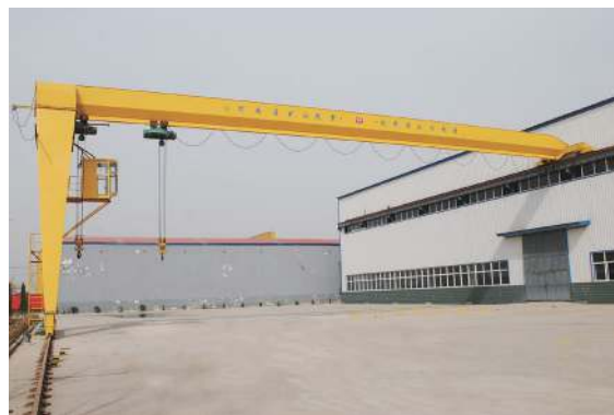
MB semi-gantry crane with electric hoist
