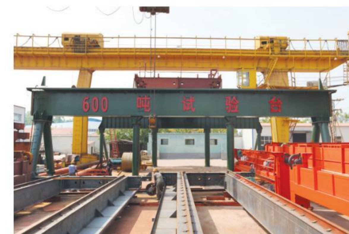
600吨桥式起重机试验台 600t bridge crane test bench
