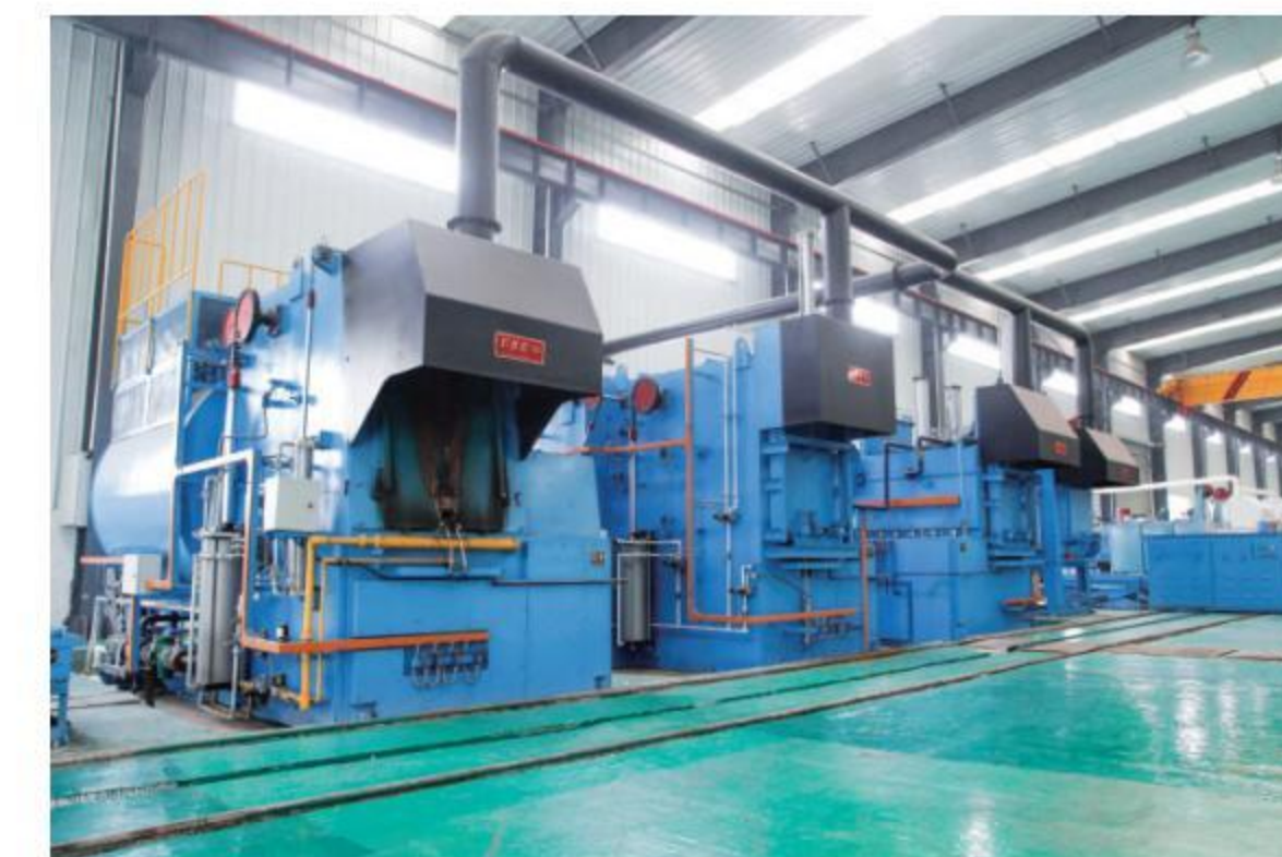
密封箱式多用气体渗碳氮化炉 Sealed box type multipurpose gas carburizing and nitriding furnace
