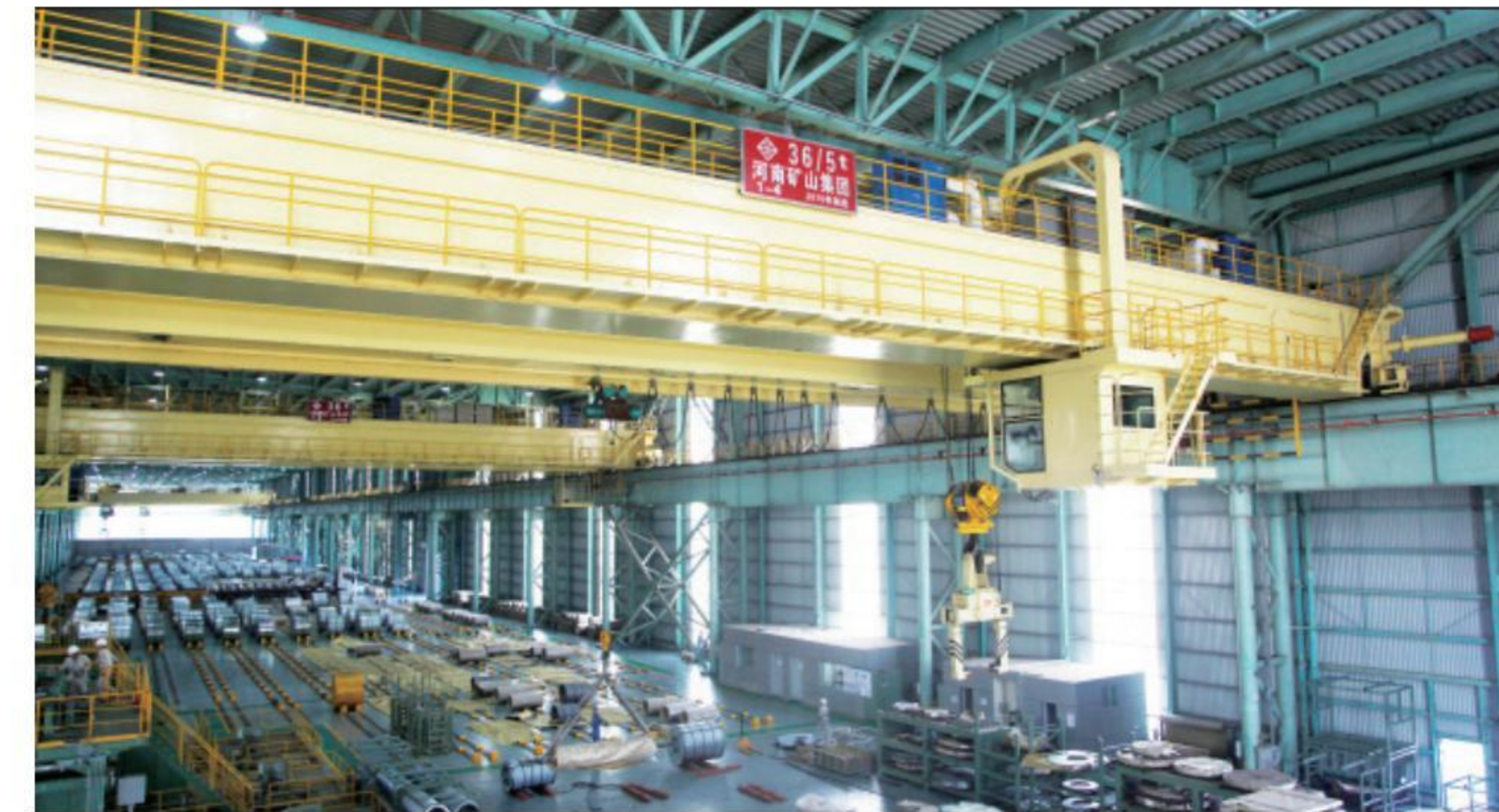
宝钢湛江项目承制的 自动化起重机 Automatic crane manufactured by Baosteel Zhanjiang project
