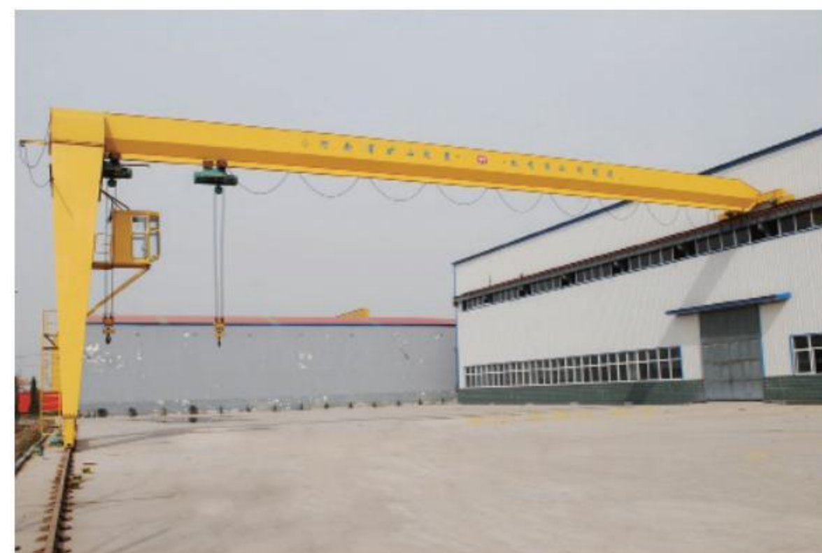
MB semi-gantry crane with electric hoist
