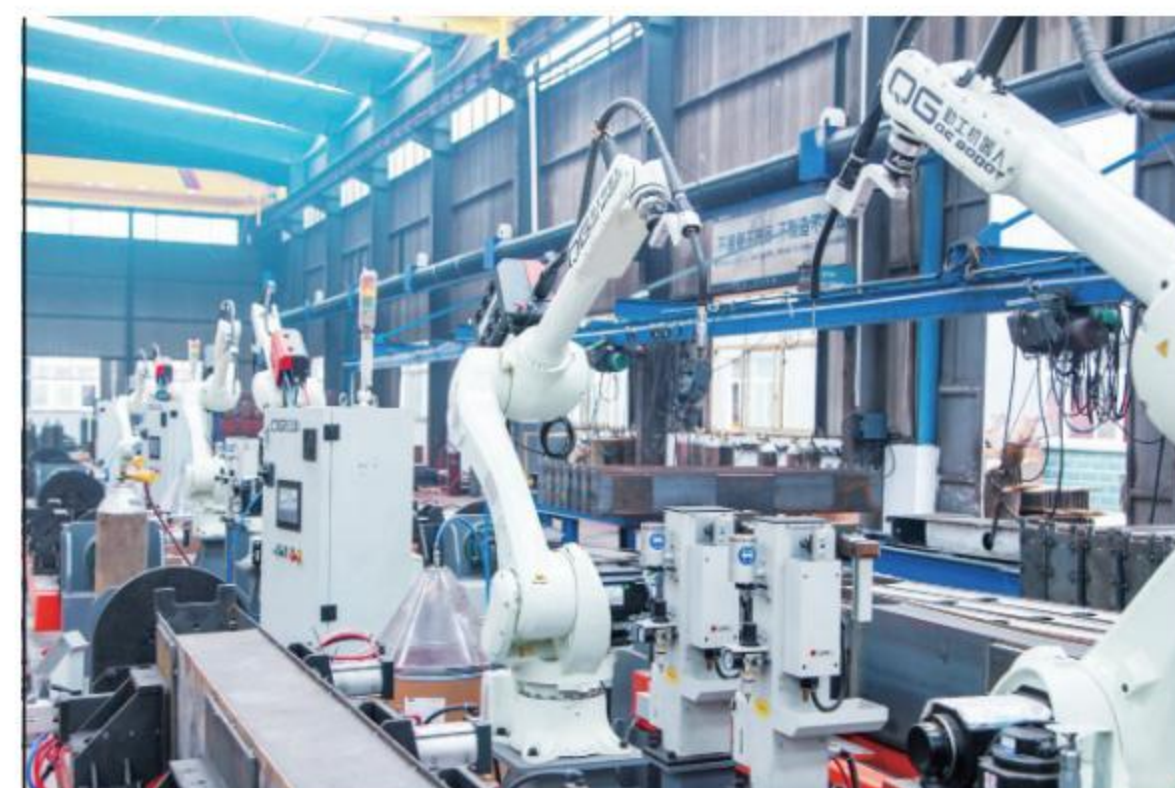
单梁端梁机器人焊接生产线 Single beam end beam robot welding production line
