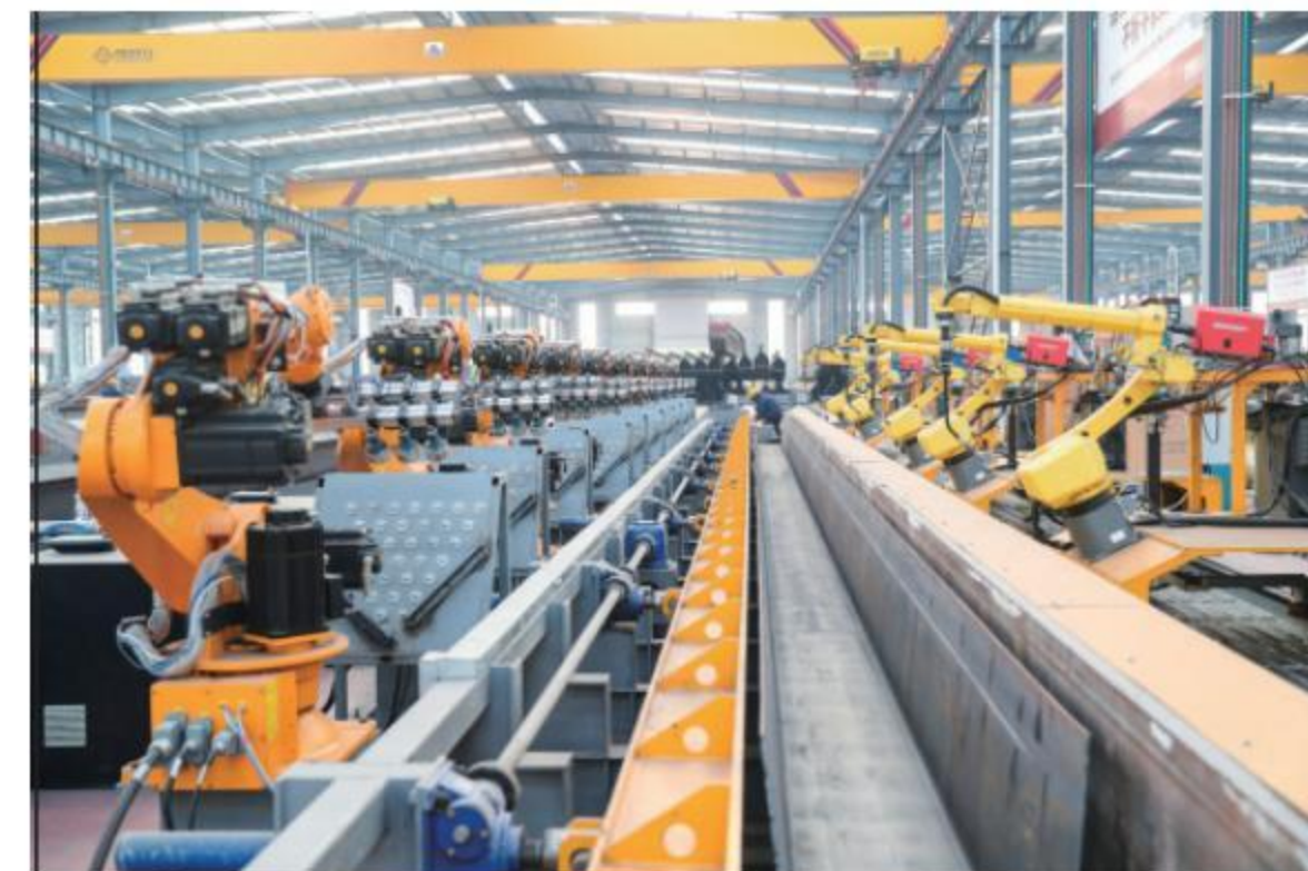
单梁筋板组装机机器人焊接生产线 Single beam rib plate assembly robot welding production line
