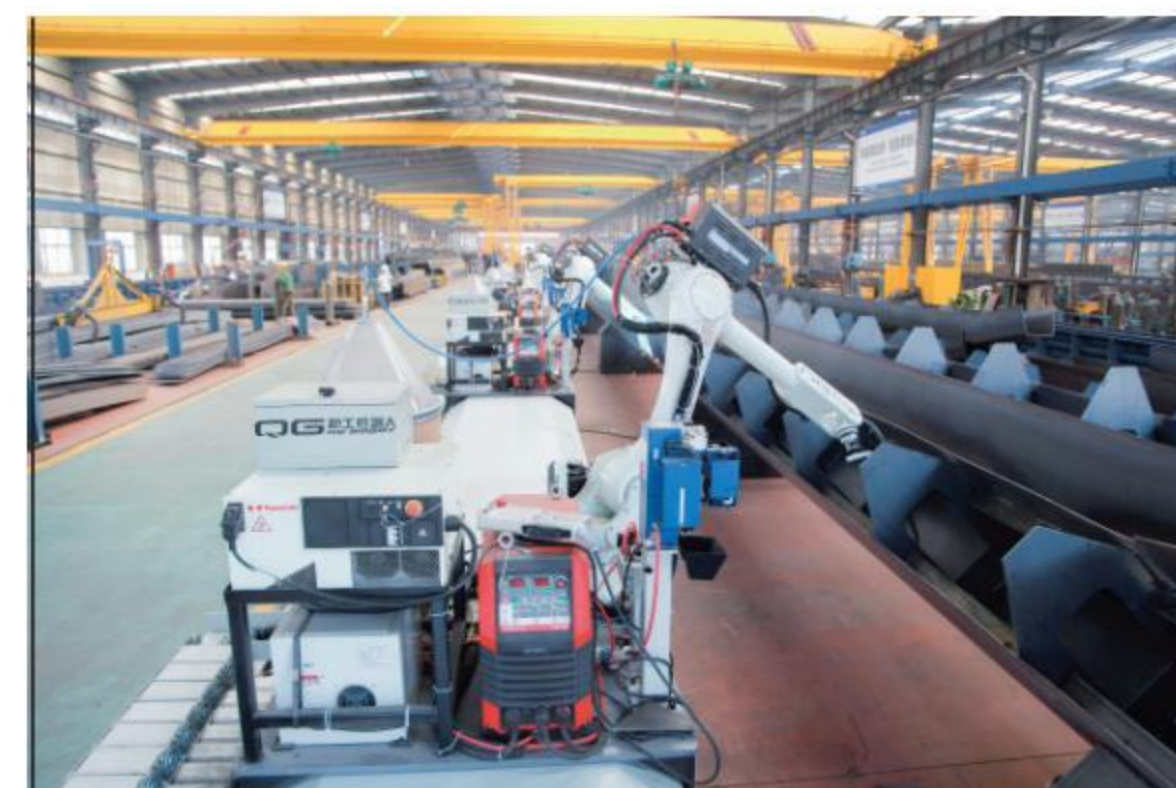
单梁主梁内缝机器人焊接生产线 Single beam main beam inner seam robot welding production line
