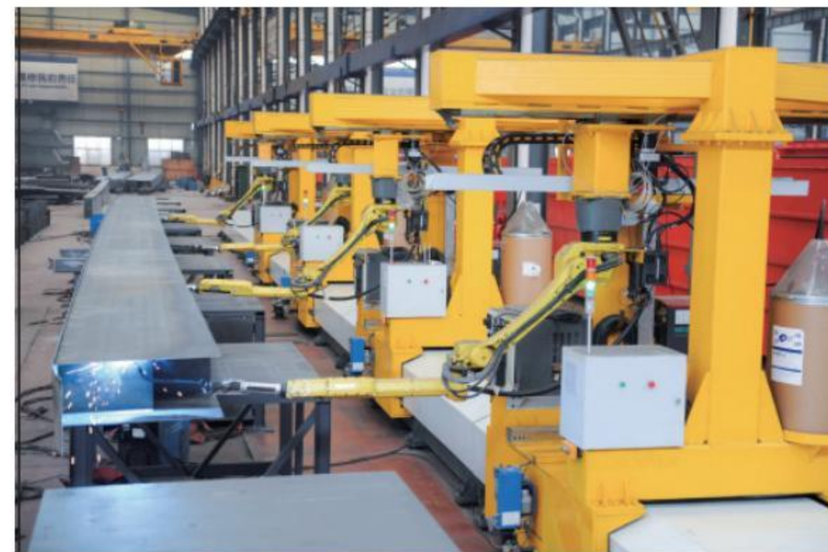
双梁主梁内缝机器人焊接生产线 Robot welding production line of double beam main beam inner seam machine
